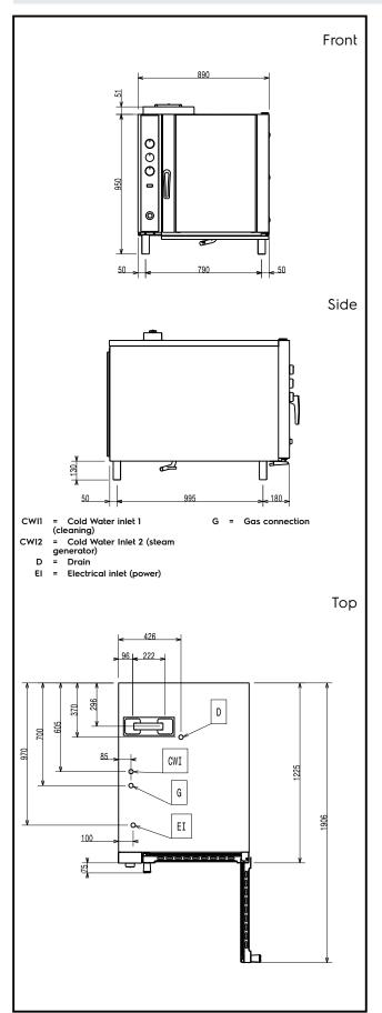
Electric Supply voltage: 260825 (EFCG12CSAS) 220-230 V/1 ph/50 Hz Auxiliary: 0.5 kW Electrical power max.: 0.5 kW Gas Gas Power: 25 kW Capacity: Trays type: 10 - 2/1 Gastronorm **Key Information:** External dimensions, Width: 890 mm 1215 mm External dimensions, Depth: 970 mm External dimensions, Height: Net weight: 154 kg 80/0 mm Height adjustment: Functional level: Basic Cooking cycles - air-convection: 300 °C
